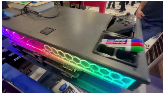
Marker storage, LEDs, and fan grilles.
