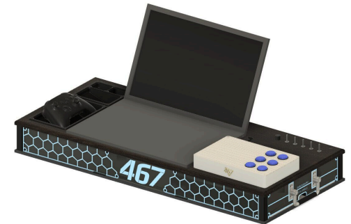
Fusion 360 model with the laptop, operator buttons, and controller tray.
